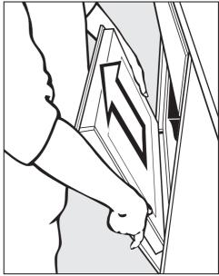
■ Hold the door on either side and pull it diagonally upwards from the hinge guides. Make sure that you lift the door off straight.
